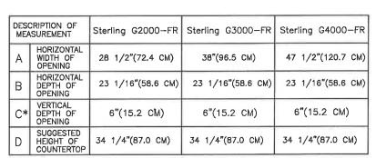
\* ADD 2" IF INSTALLED WITH COMBUSTABLE MATERIAL UNDER GRILL
